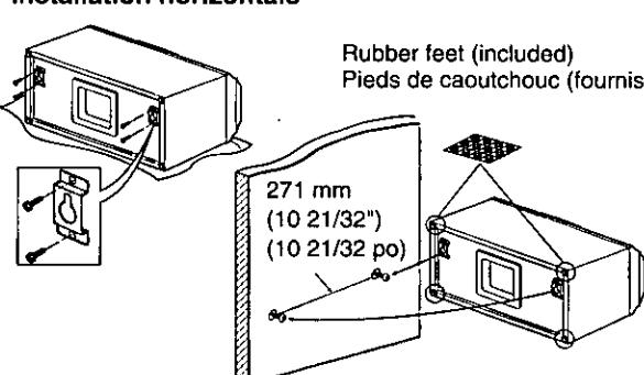
**Note** The surface you attach the speakers to must be able to support over 13 kg (28.7 lb.).
