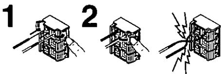
(Connection to the speakers)/(Raccordement aux enceintes)
