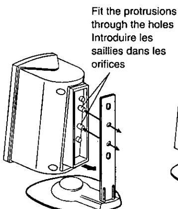
Fit the protrusions through the holes
